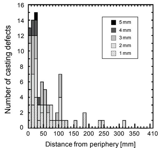
**Fig. 5 Distribution of casting defects detected by MT from the periphery to the center of the bottom surface**
