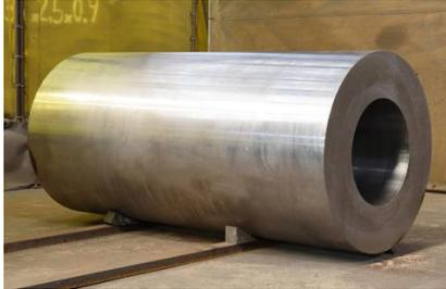
**Fig. 3 Photograph of the fabricated full-scale cast steel overpack with 1750 mm in length and 820 mm in diameter**
