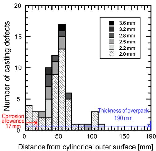
Fig. 7 Distribution of casting defects detected with UT from the outer surface to the inner surface of the cylindrical body
