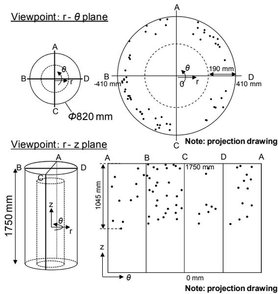
Fig. 6 Results of UT (inside defect testing)
