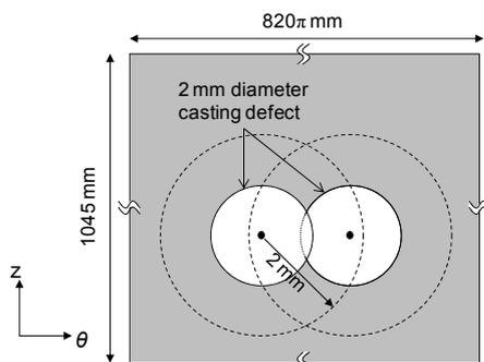
**Fig. 11 Schematic diagram of overlapping of casting defects in the thickness direction (Note: the axes corresponds to Fig. 6)**
