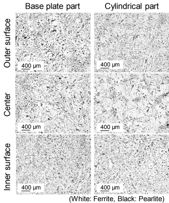
Fig. 8 Microstructures at six sampling positions
