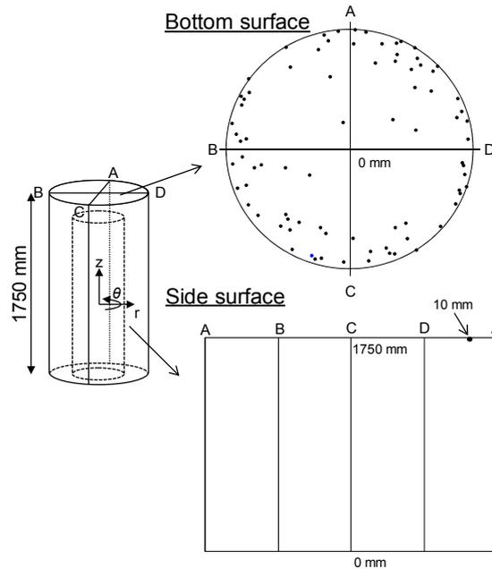
**Fig. 4 Results of MT (surface defect testing)**
