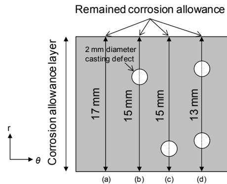
**Fig. 10 Schematic diagram showing a state in which the required corrosion allowance is not ensured due to casting defects (Note: the axes corresponds to Fig. 6)**
