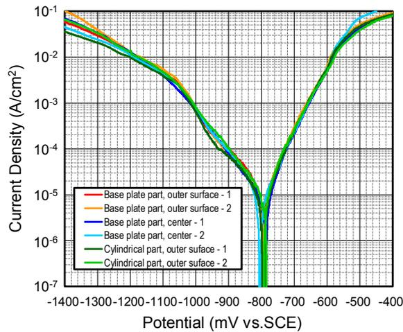
**Fig. 9 Anodic / cathodic polarization curves in the synthetic sea water**
