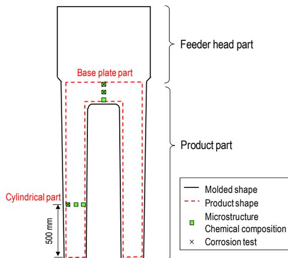
**Fig. 2** Casting configuration and sampling positions for microstructural observation, chemical composition analysis and corrosion test
