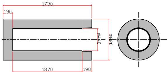
**Fig. 1** Dimensions of fabricated overpack (mm)
